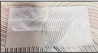
Transparent plexiglass simulates a tile laid in thinset mortar applied with a curving motion of the notched trowel. Note the inability of the ridges in the mortar to collapse due to nonuniformity of the troweling.
