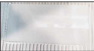
Transparent plexiglass simulates a tile laid in thinset mortar applied with a one-directional motion of the notched trowel. Note the ideal embedment of the tile due to the ease of mortar ridge collapse.
